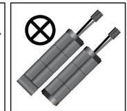
Do not use a 6-cell 7.2V battery in combination with a 7-cell battery 8.4V pack.
