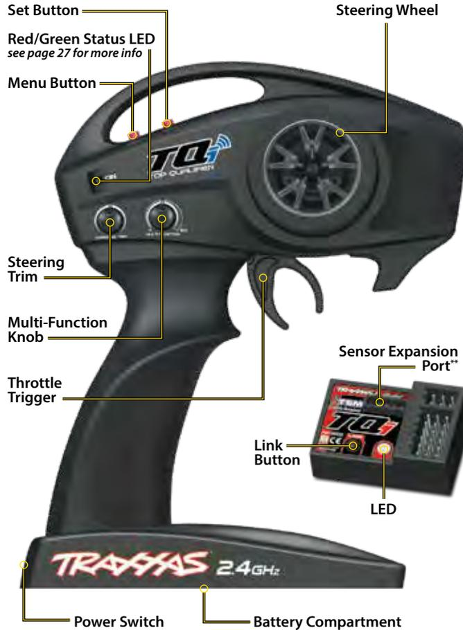
\*\*Accessory sensor expansion port for use with the Telemetry Expander Module (see Traxxas.com for more information).
