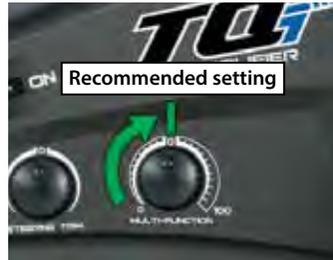
Turn the knob clockwise to increase assistance; turn the knob counterclockwise to decrease assistance. Turn the knob counterclockwise to its stop to turn TSM completely off.
