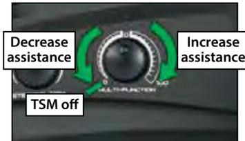
**Note:** TSM is deactivated automatically when driving in reverse.
