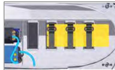
**Battery Packs Aft:** Smooth water and calm winds may allow you to move the battery packs rearward in the hull to allow the bow to ride higher and increase Spartan SR's speed. Positioning the batteries farther aft increases the likelihood of the boat blowing over at speed or becoming unstable.
