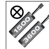
Do not mix battery capacities. Use two batteries with the same capacity.
